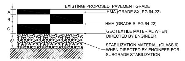
NOTE 1: IF PATCHING, AREA TO BE PATCHED SHALL BE SAWCUT TO THE FULL DEPTH OR CUT BY A METHOD APPROVED BY THE ENGINEER WHICH LEAVES A VERTICAL FACE ON THE EXISTING PAVEMENT AND NO DEFORMATION OF THE SURFACE AT THE CUT. APPLY TACK COAT TO CUT FACE.
