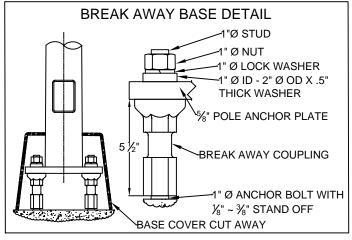
WHEAT RIDGE 20' ROUND TAPERED STEEL POLE WITH GE ERL1, DEEP ABS BASE COVER, AND BREAK AWAY COUPLINGS
