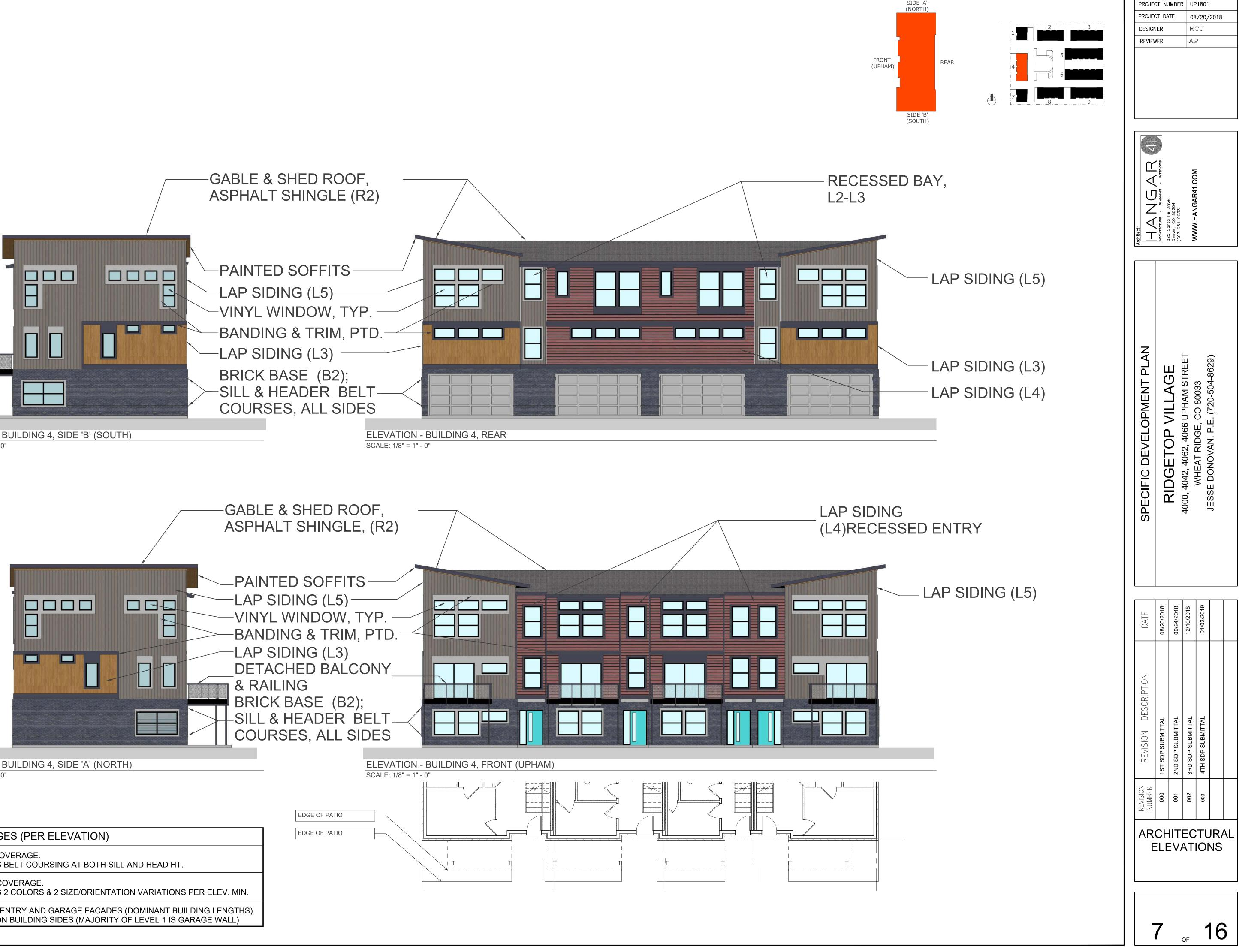
ELEVATION - BUILDING 4, SIDE 'A' (NORTH) SCALE: 1/8" = 1" - 0"
