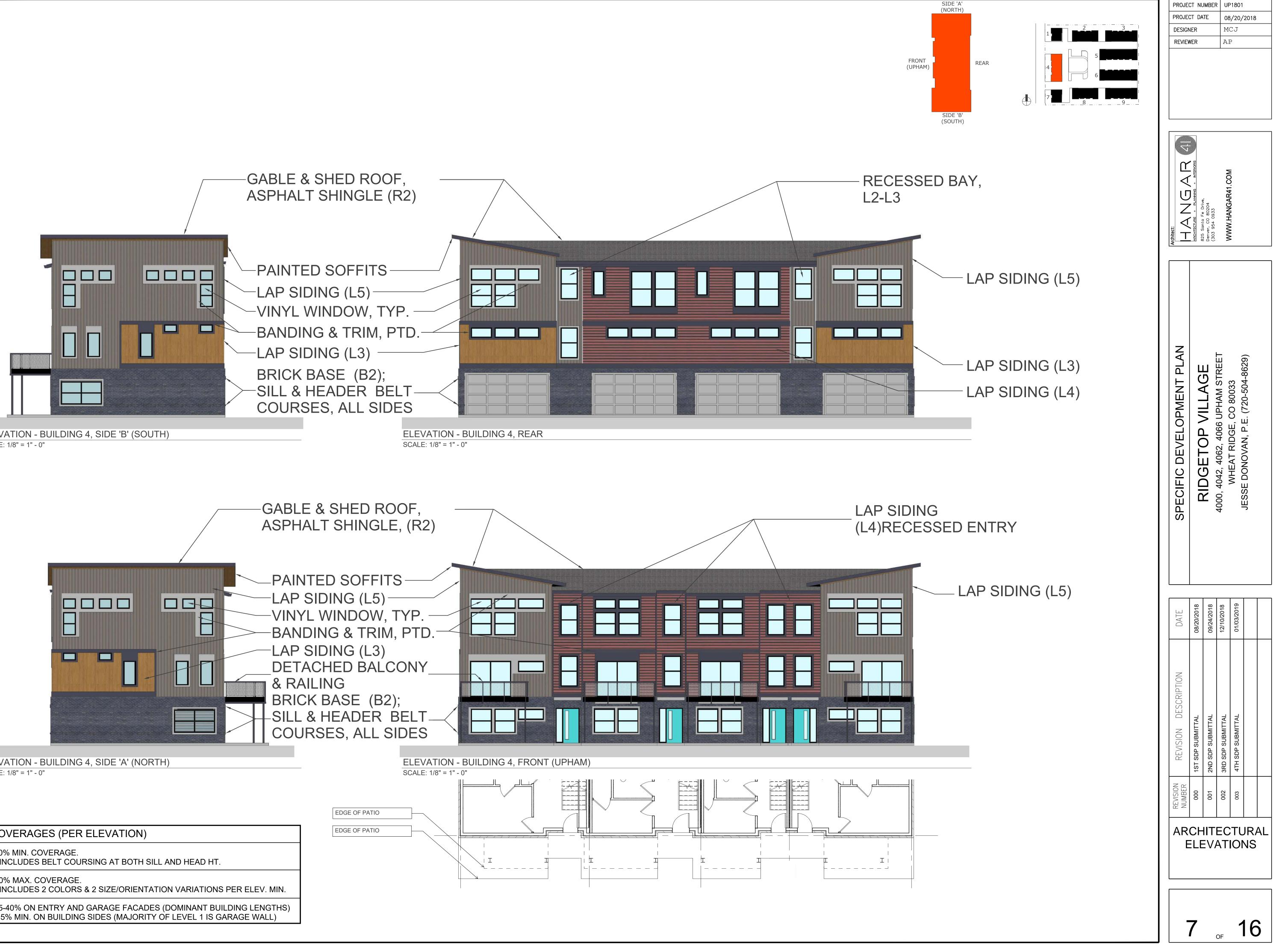
ELEVATION - BUILDING 4, SIDE 'B' (SOUTH) SCALE: 1/8" = 1" - 0"
