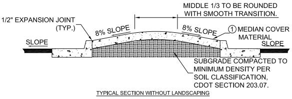
(1) MEDIAN COVER MATERIAL DESIGN & COLOR TO BE APPROVED BY CITY ENGINEER PRIOR TO CONSTRUCTION.
