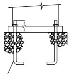
1/2" O/D X 18" HOT DIP GALVANIZED L-TYPE ANCHOR BOLTS (4 PER POST). ATTACHING HARDWARE SHALL BE STAINLESS STEEL WITH STAINLESS STEEL ACORN CAPS
